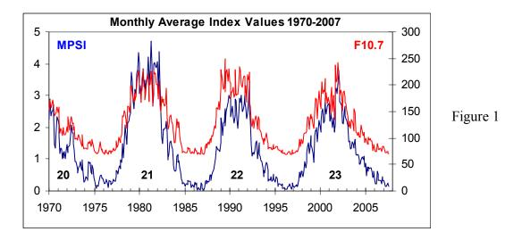
In fact, as Figure 2 shows, the MPSI is 35% too high before the magnetograph upgrade in 1982.5. The MPSI is proportional to the part of F10.7 flux above 63.5 sfu. We find that
